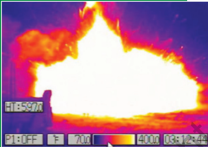
Infrared view of compressed hydrogen cylinder failure
