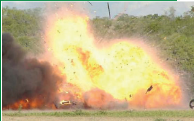
Catastrophic failure of a compressed hydrogen cylinder installed on a vehicle
