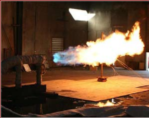
Calibration of SwRI's jet-fire apparatus
