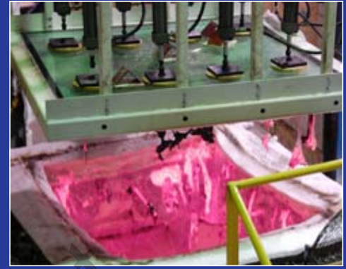
Fire resistance test of floor/ceiling assembly
