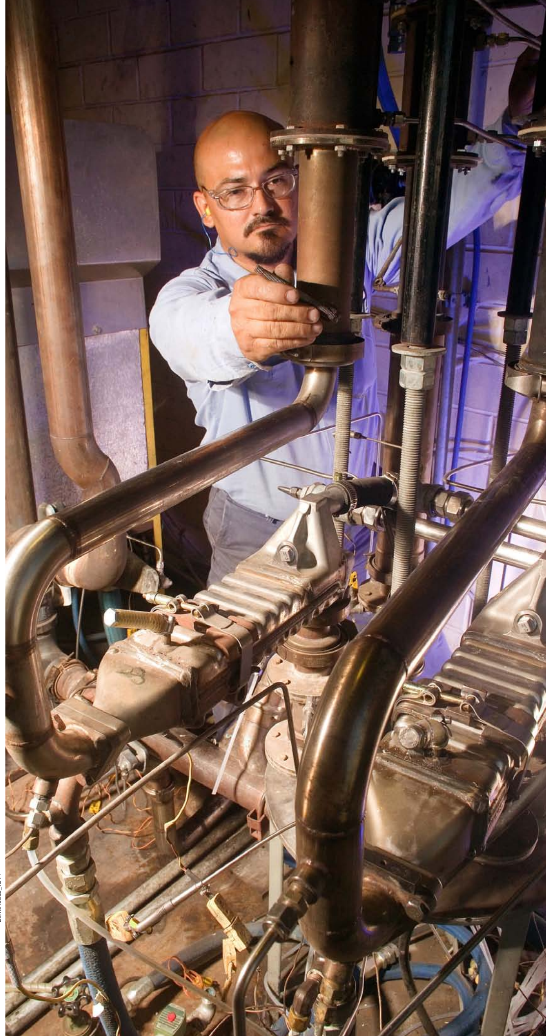
Accelerated EGR cooler thermal cycle durability testing for engine manufacturers and component suppliers
