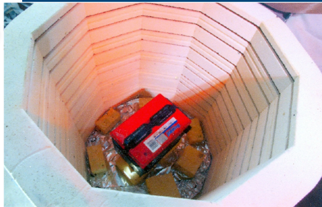
High-temperature battery testing in SwRI's 7-ft 3 capacity kiln may include temperatures higher than 2300°F.
