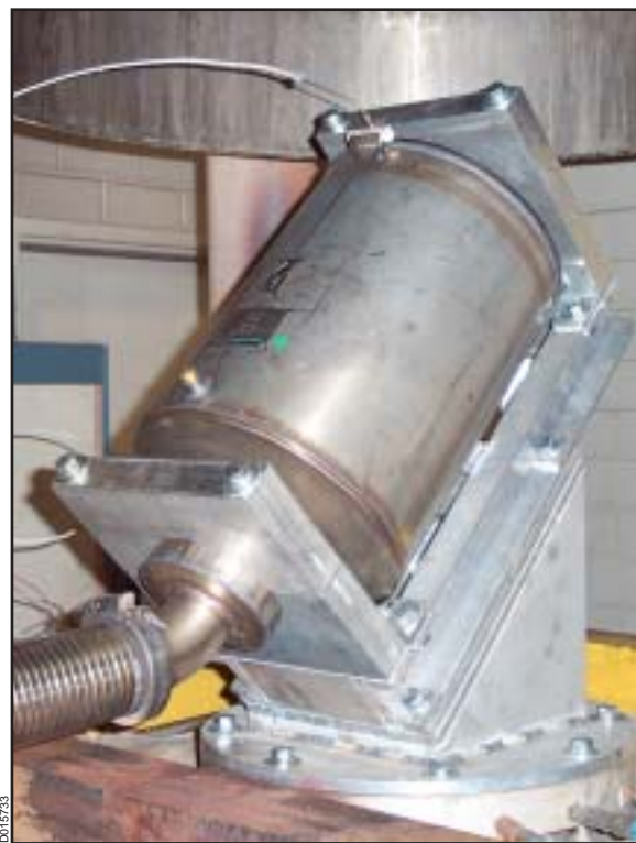
Example of fixture for mounting large-engine catalytic converter at 45° angle.
