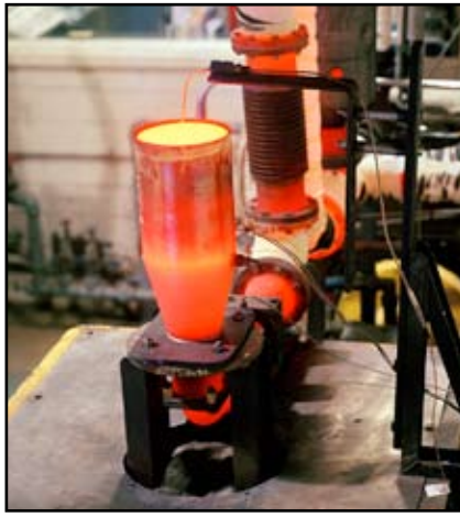
Automotive catalytic converters undergo full-flow thermal cycle and hot vibration testing to ensure durability for the vehicle life. Catalyst substrates and support systems are evaluated under accelerated test conditions following OEM, component supplier, or SwRI test protocol.
