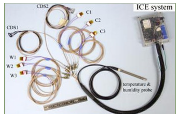
ICE system with 3 wetness sensors (W), 2 coating degradation sensors (CDS), 3 corrosivity sensors (C), and a dual probe for temperature/humidity.
