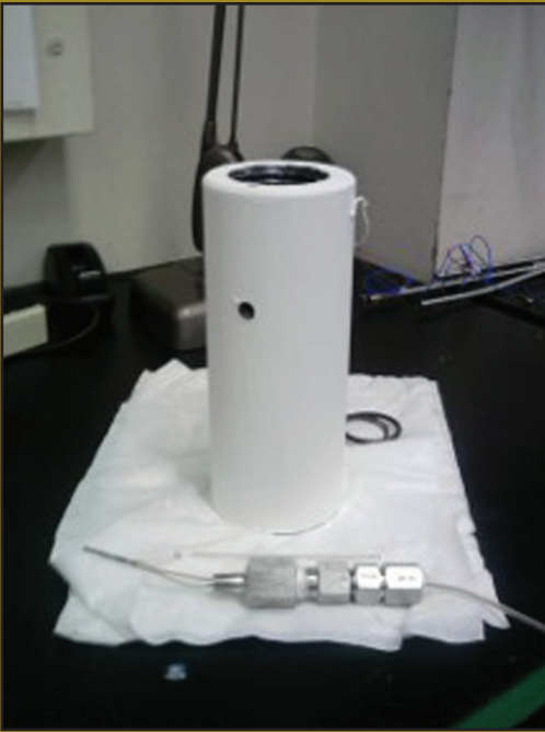
High-pressure adiabatic test fixture for measurement of specific heat
