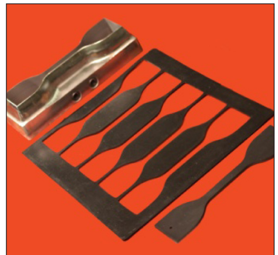
Thin polymeric and rubber specimens are 'stamped out' of flat plates with certified cutting dies for various standardized tensile specimen shapes and sizes.
