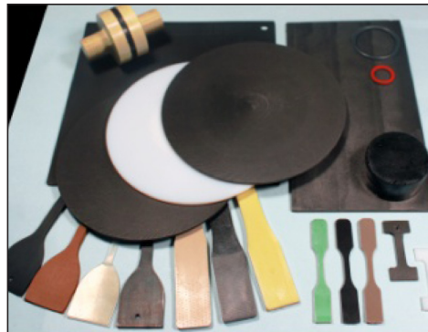
SwRI evaluates the effect of HPHT toxic gas or fluid environments on the mechanical properties of different types of polymeric compounds.
