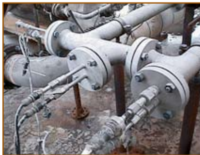
SwRI developed and implemented multi-electrode array sensor (MAS) probes to monitor localized corrosion of chemical process system components in real time.
