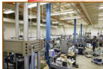
SwRI designed and constructed a specialized test system to enable examination of microbially influenced corrosion of pipelines at elevated pressures to explore possible telltale fingerprints associated with biotic corrosion.
