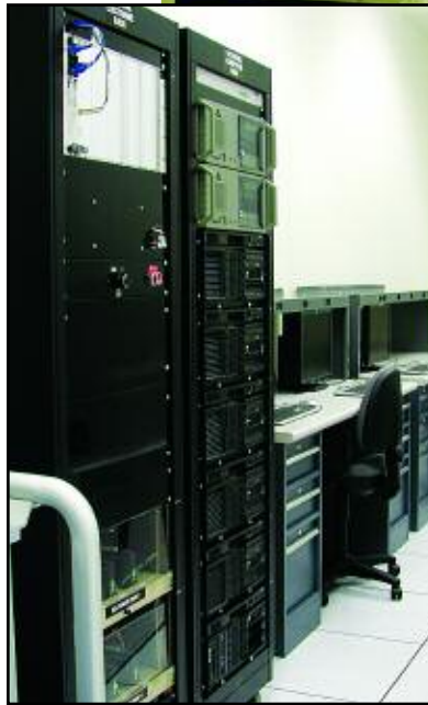
The FTD student and instructor stations are housed in an air conditioned enclosure. External equipment racks (left) house computers, power supplies and electronic equipment.
