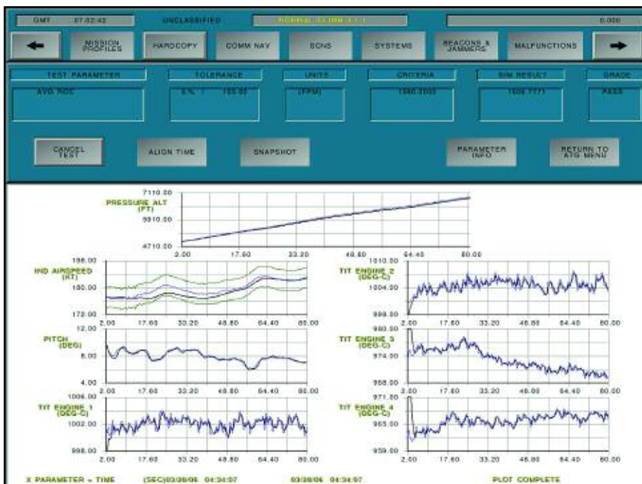
The certification process includes the comparison of recorded C-130 aircraft data with simulator data. The simulator pilot flies the same maneuver used in the aircraft; in this case, a normal climb after take off. Notice that the simulator airspeed (black line) stays within the tolerance bars.
