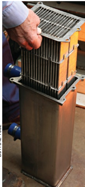
EGR coolers are a key component to enabling high efficiency. Exhaust gases flow through the cooler, which is bathed in engine coolant.
